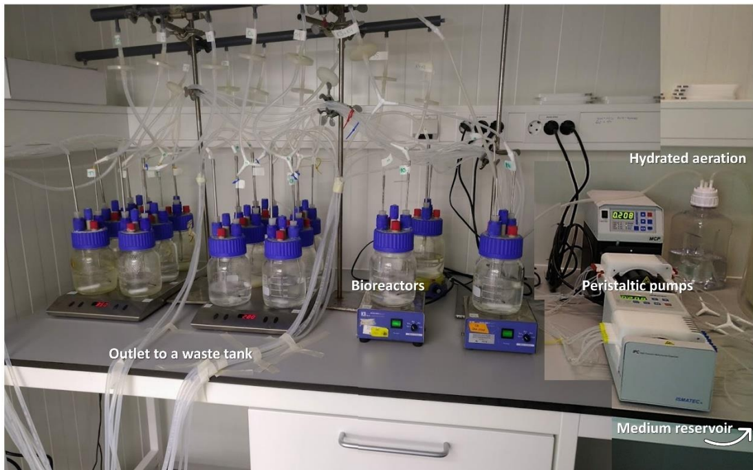
Figure 5: The experimental setup. Bioreactors were supplied with media from a media reservoir by two peristaltic pumps. The medium was mixed with hydrated air and delivered through the silicone tubes.
