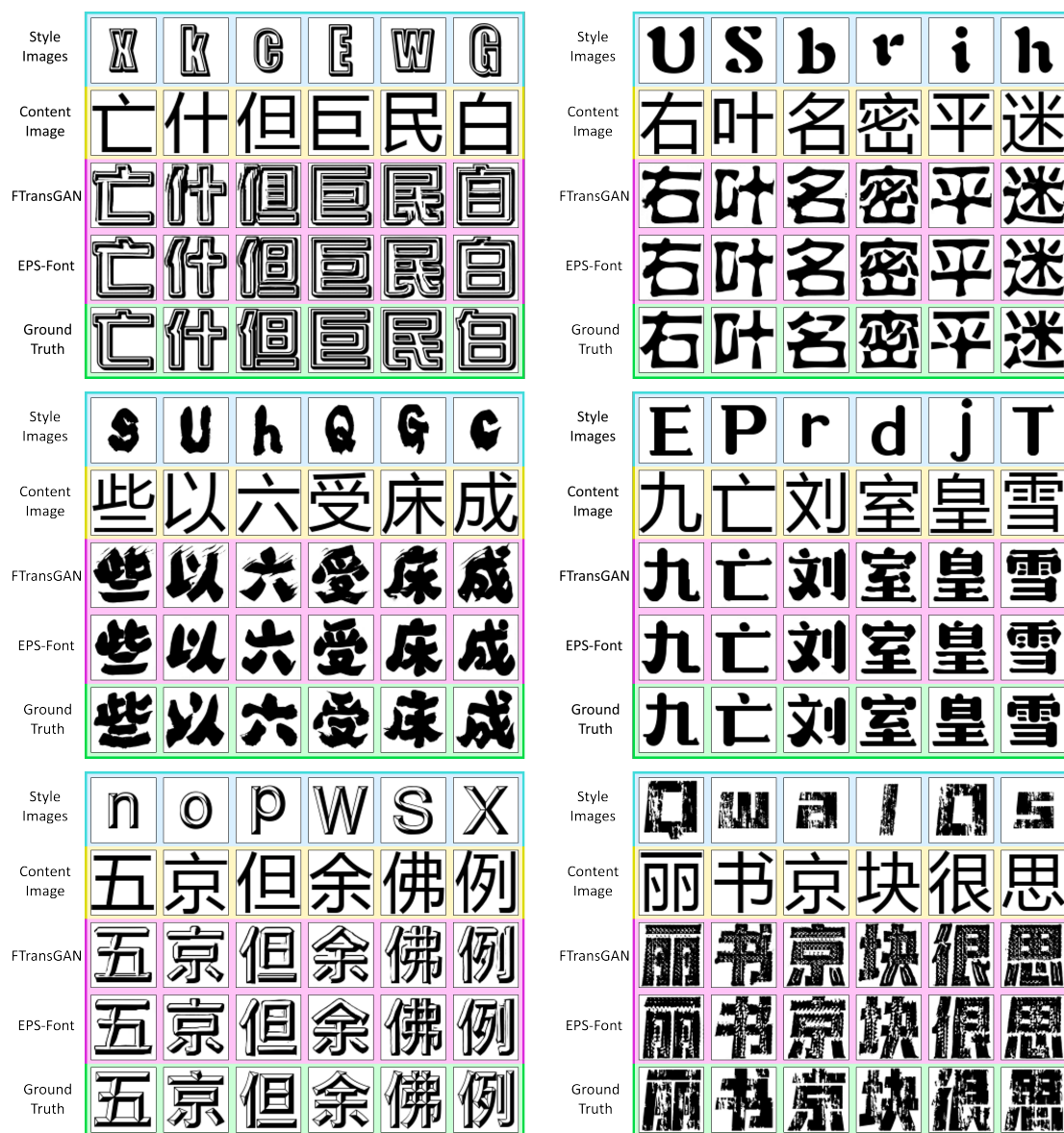
Figure 6.2.: Generated examples from FTransGAN and EPS-Font. Both models are able to extract the style well. However, the generated images from EPS-Font are often sharper than the generated images from FTransGAN.
