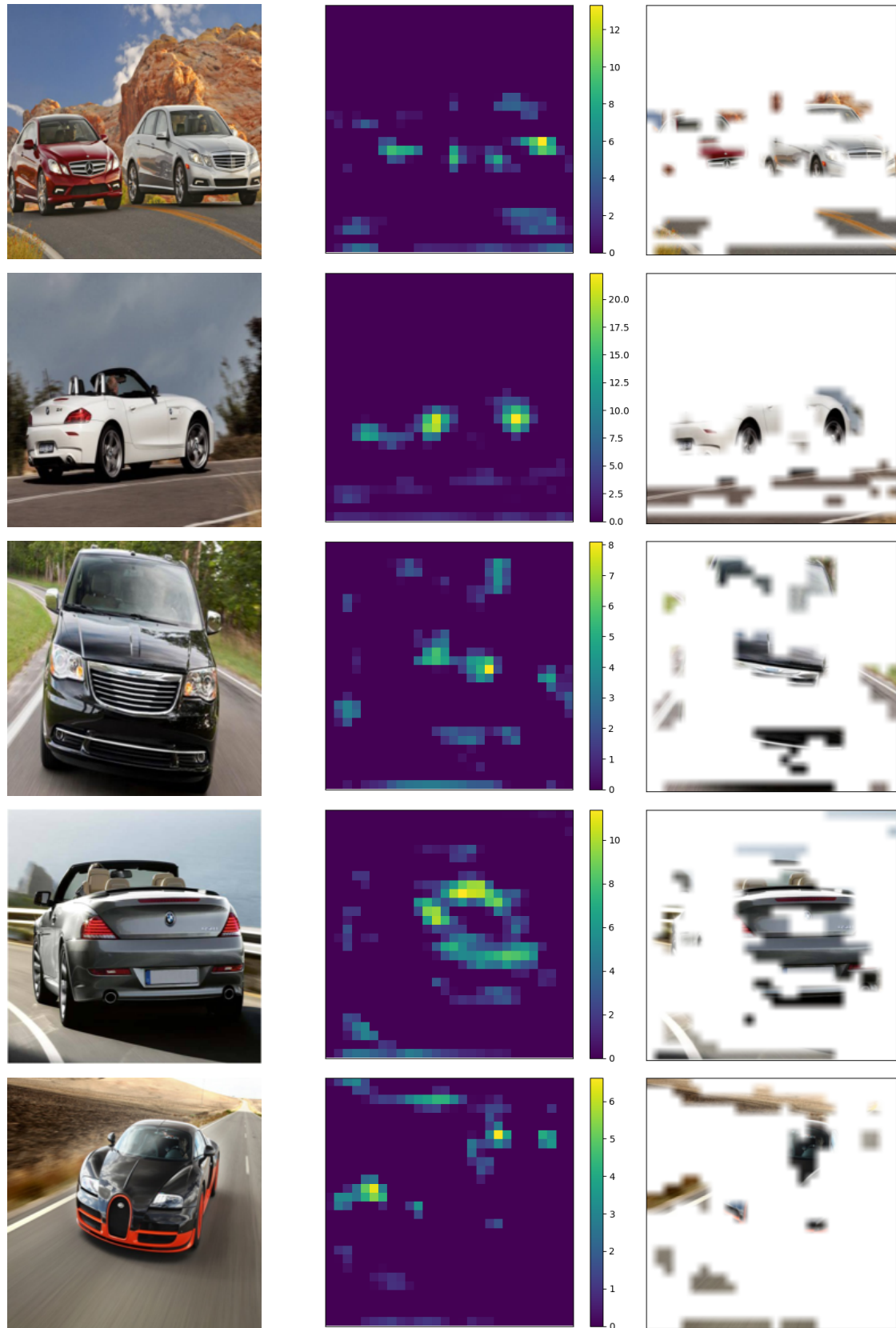
Figure 6.7: Example of filter 429 from Conv4-3 of VGG16 that activates for car parts and road surface markings. The road line activations are usually weaker but still appear. Each row is one example, where the first column is the original image, the second column the ReLU activated feature map, and the third is the original image with an alpha mask that is one where the interpolated feature map is active and 0 everywhere else.
