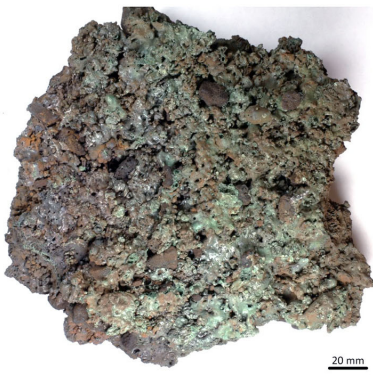
Fig. 2—Slag infiltrated charge sample at top of the furnace charge taken from a FeMn furnace (left picture) showing low alkali binder phase (right). [4]
