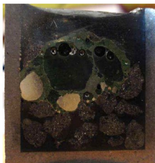
Fig. 6—FeMn-production: Slag viscosity during cooling adapted from Ref. 1 (left) and example of reduced slag from Comilog ore at 1600 °C [21] (right).
