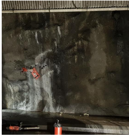
Fig. 3: Six shotcrete cores extracted in the Hitra tunnel at chainage 3+090 (approximately in the middle of the tunnel). The extracted cores are shown in Fig. 33.
