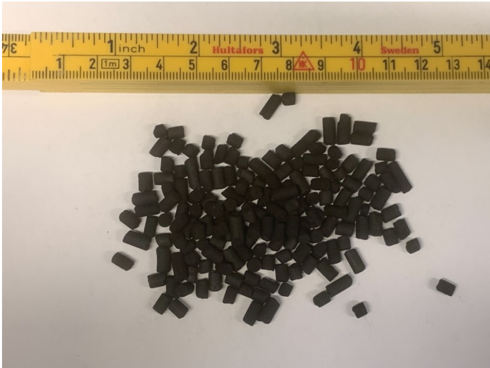
Figure 2: Used PAC at Equinor VOCs experiments
