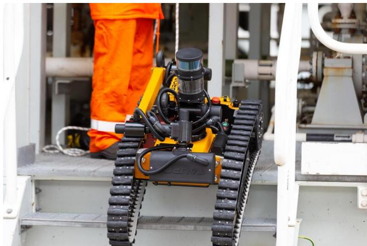
**Figure 1.1:** An autonomous inspection robot created by Equinor which has been deployed to an offshore platform. Source: [2]
