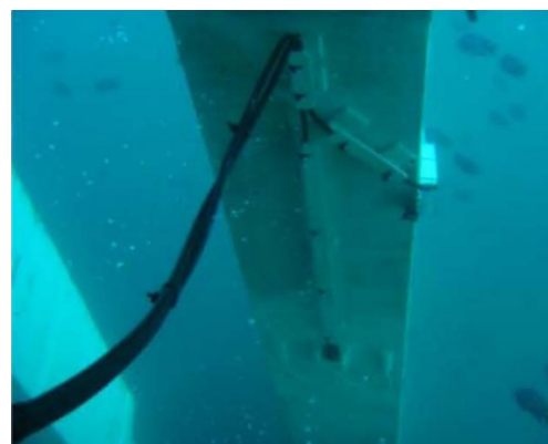
(b) Direct load monitoring with electrical strain gauges. Courtesy: Hageman et al. (2019)
