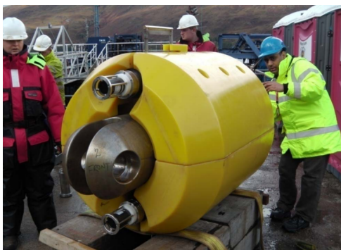
(a) Inter-M Pulse H-link for direct tension measurement. Courtesy: PULSE mooring monitoring
