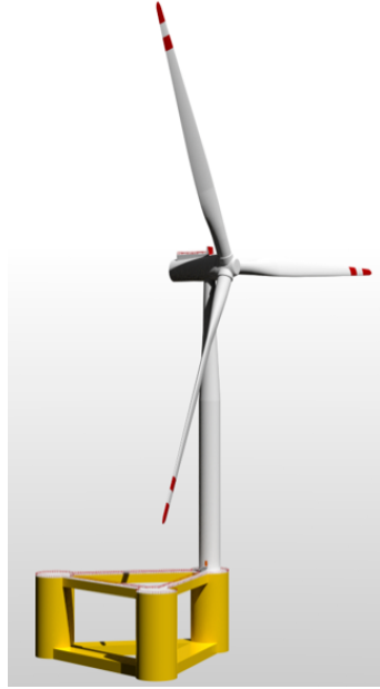
Figure 4.3: INO-WINDMOOR 12 MW FWT concept (Souza et al., 2021)
