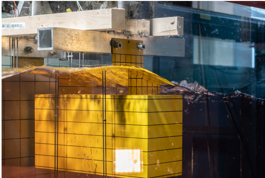
Figure 6.8: Perspective view of incident wave with significant wave overtopping of the pontoon.
