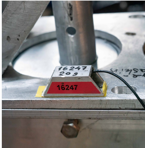
Figure 6.14: Accelerometer installed on top of the rig.
