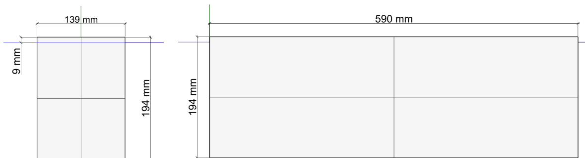
Figure 6.1: Model for testing in Ladertanken. Model scale of 1:36. The horizontal blue line marks the mean water level.
