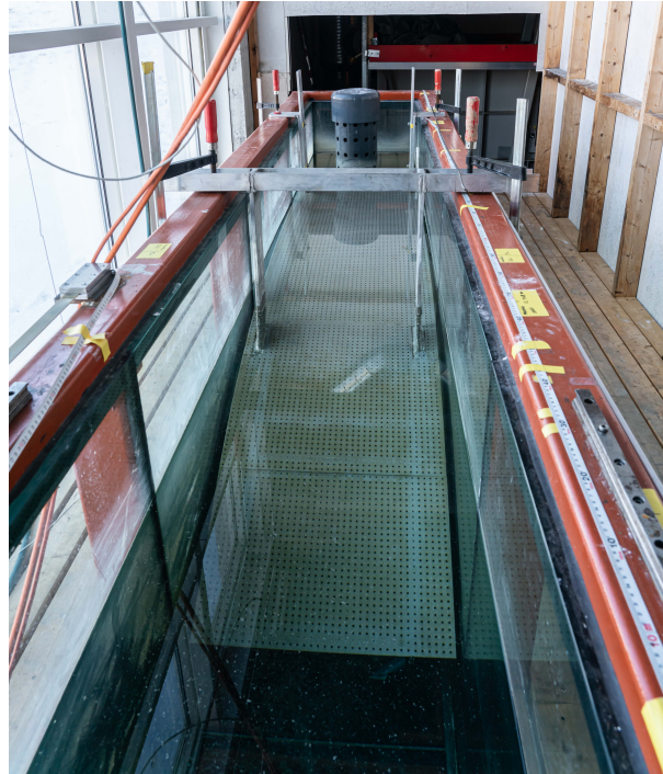
Figure 6.6: Parabolic beach installed on the opposite side of the wavemaker. The beach is made of a perforated plate which was about 0.5 cm below the free surface at the top point.
