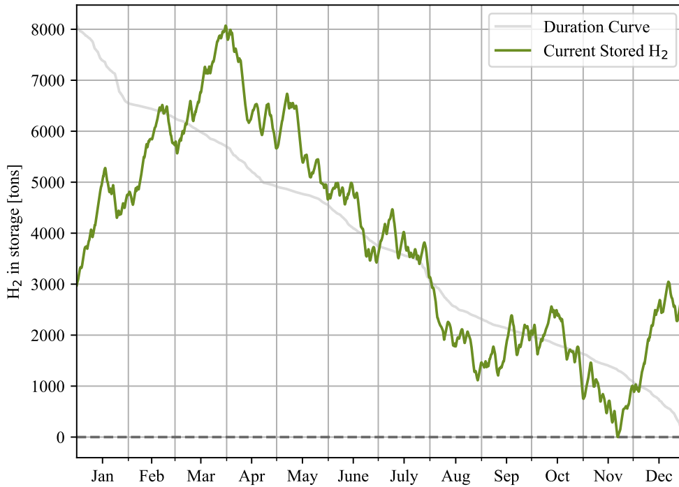
Figure 6.1: Storage status a hydrogen storage connected to a modelled offshore wind and hydrogen power plant, both of 1400 MW capacity. This case have a constant delivery to shore every hour in the whole year. The delivery to shore was 15.7 tons each hour.
