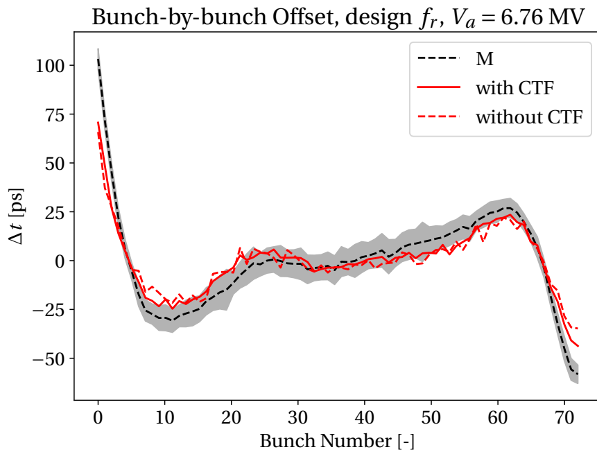
Figure 3.19: Bunch-by-bunch offset of the first batch in a simulation with V_{\text{ant}} = 6.76 MV and TWCs with their original design resonant frequencies. The full red trace is with the cable transfer function (CTF) and the dashed red trace is without.
