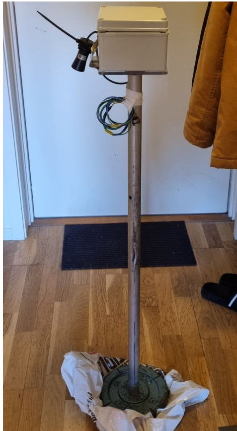
Figure 4.1.14: Image of the final container and stand for the embedded hardware.
