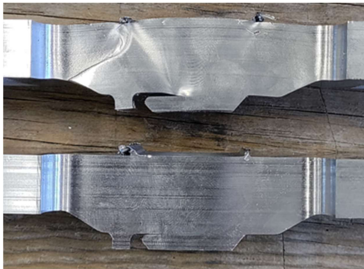
Figure 55: Horizontal bowing in specimen after testing
