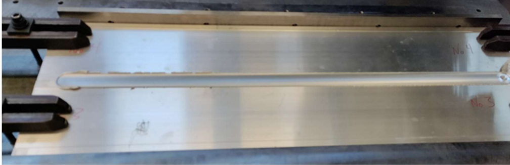
Figure 17: Gapless weld of 17 mm thickness
