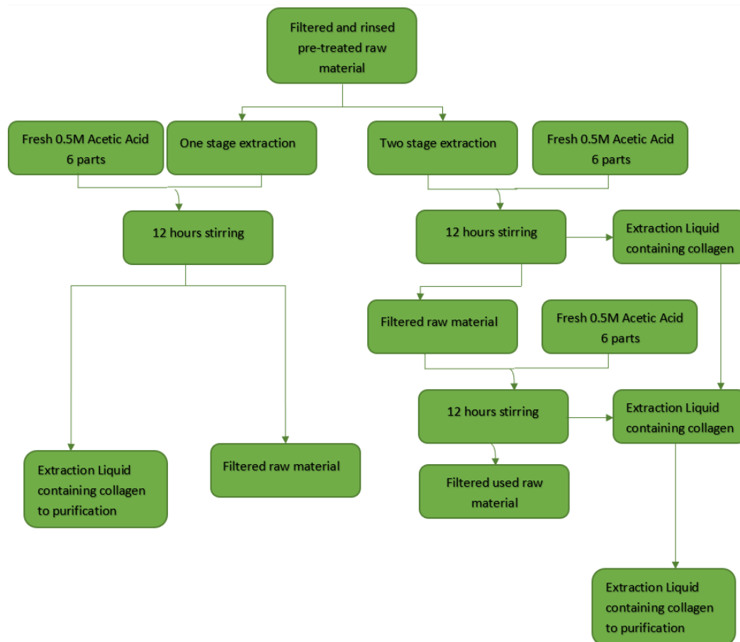
Figure 2.2: Flowchart of how the collagen is extracted, including both one step and two step extraction with acetic acid. For the two step extraction the two extraction liquids are combined.
