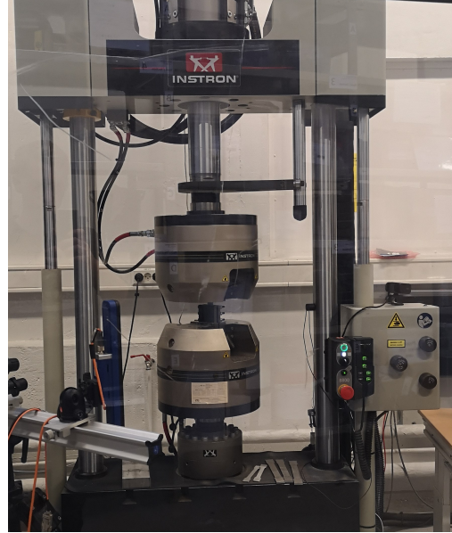
Figure 3: The Instron Machine Used During Tensile Testing for Non-Saturated Specimens
