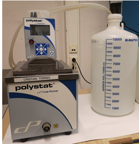
Figure 2: Water Bath on the Left with Vessel Filled with Distilled Water and Specimens on the Right
