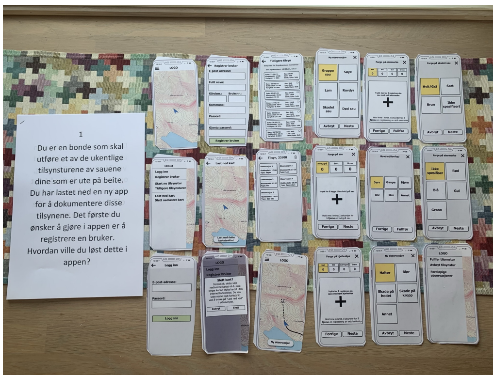
Figure 39: How the user test for the mobile application paper prototype was set up. The "wizard" changes the active paper sheet whenever the test user makes an interaction. The user also always has their current test task visible in front of them.
