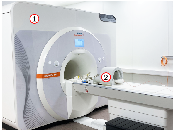
Figure 4.1: (1) Siemens MAGNETOM Terra MR scanner. (2) Nova 1Tx/32Rx head coil.
