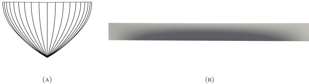
FIGURE 4.5: Body plan (A) and visualisation (B) of the Wigley model.
