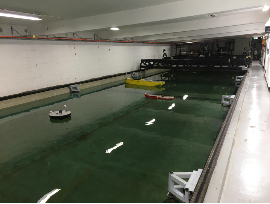
Figure 3.5: The CSS, CSE1 and CSAD deployed in the MC lab basin
