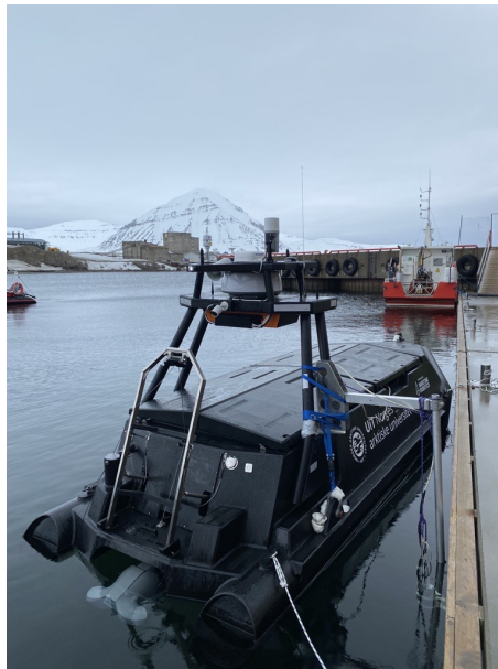
Figure 4.7: Mounting of USBL modem on the ASV in Ny-Ålesund, leading to asymmetric drag on the hull.
