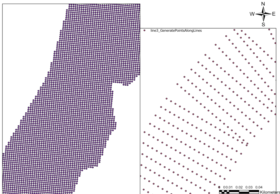
Figure 3.3: Full raster point(Left panel) and cross-sectional point line(right panel) along the river
