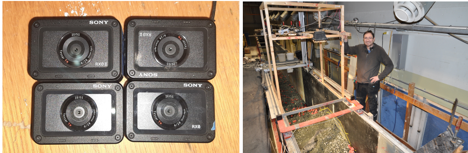
Figure 3.7: Sony Camera RX0/ROXOII on the left and wooden frame for camera stand on right
