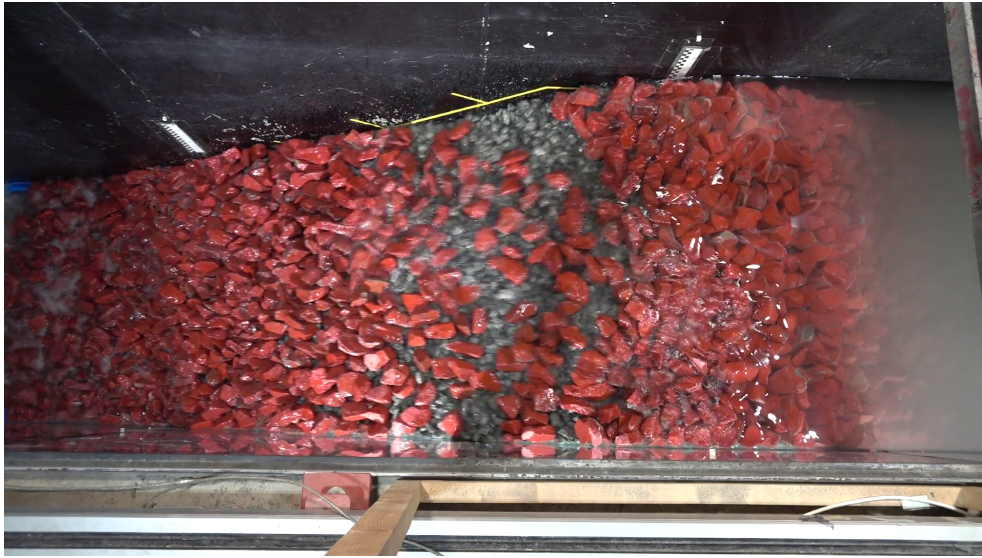
Figure 4.2: Sliding in placed riprap due to overtopping, t=25 s
