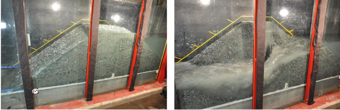
Figure 5.3: Left side- Dam model before breaching with pilot channel on the top Right side-Dam model after breach progress around pilot channel
