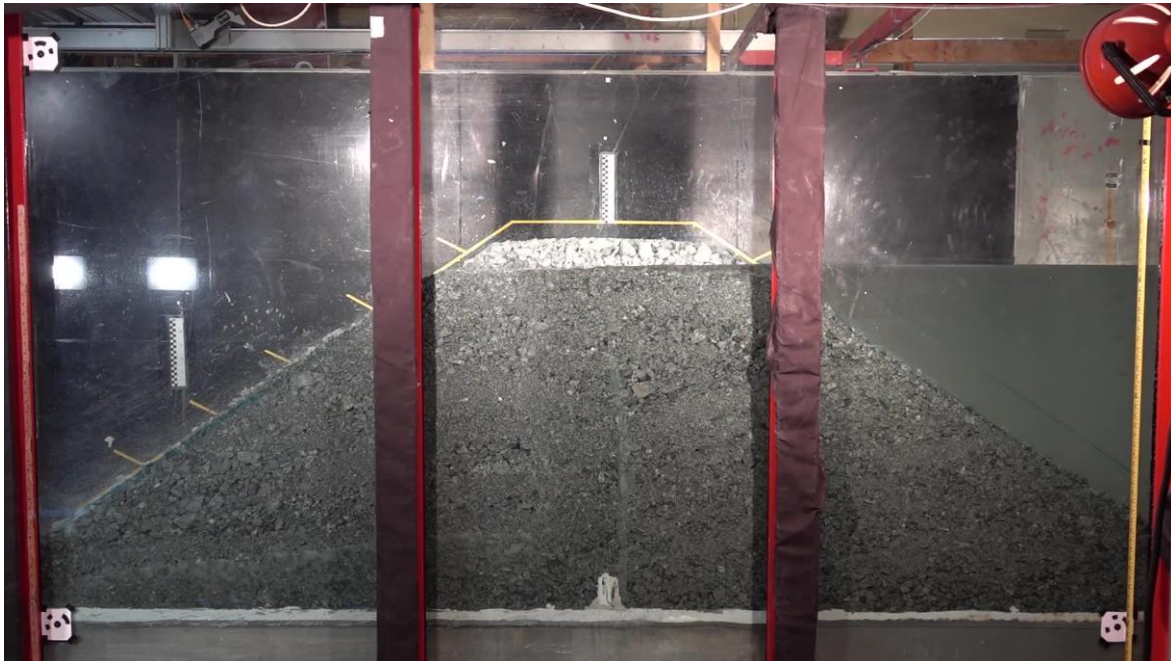
Figure 3.6 Water just overtopped on rockfill core dam
