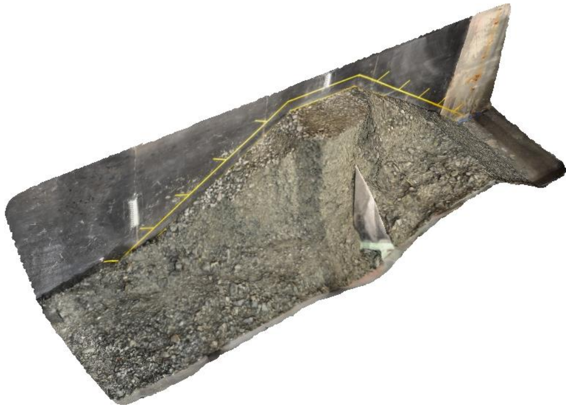
Figure 4.8: Three dimensional model of M15 after breach
