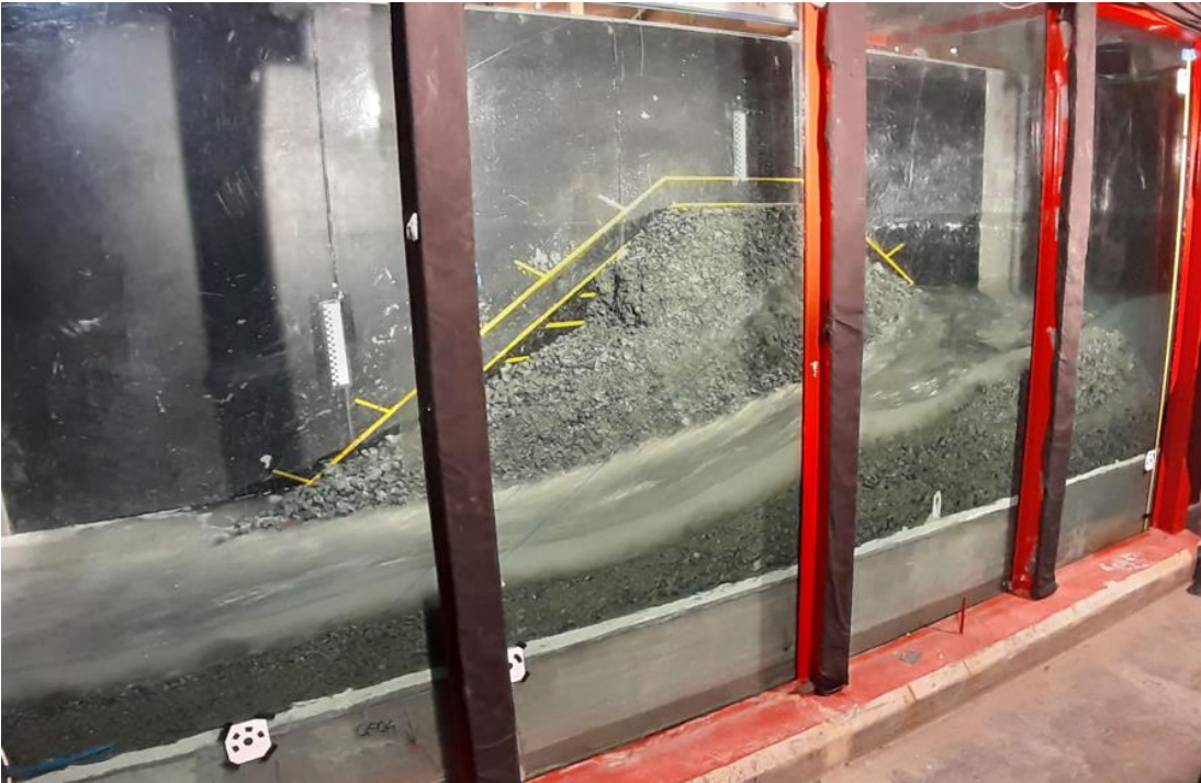
Figure 3.9: Rockfill dam without core final breaching view
