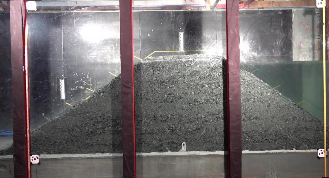
Figure 3.8 Rockfill dam without core with excess throughflow
