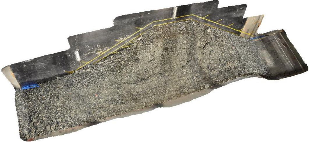
Figure 4.16: Three dimensional model of M17 after breach
