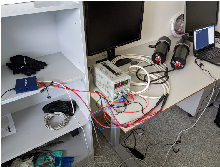
(a) The modems were connected to a computer using a switch. A power source was used to provide power to the modems during longer periods of time.
