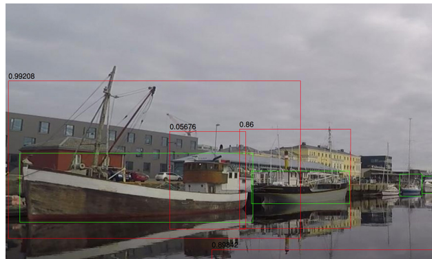
Figure 1.1: False positive maritime vessel detection.
