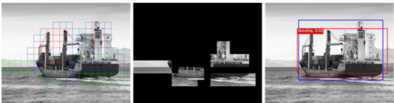
Figure 4.25: Sample of wrongly classified object, k = 100
