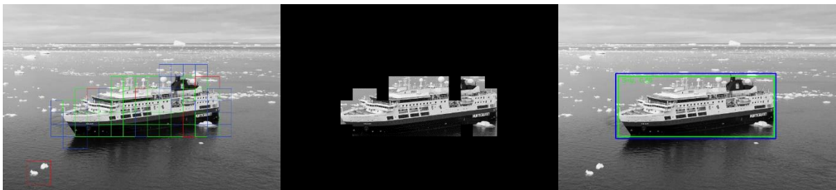
Total number of positive patches: 28 Total number of negative patches: 5 IoU ship: 0.9015066065098292
