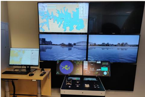
**Figure 5.** Research training bridge at the Department of the Ocean Operations and Civil Engineering at NTNU in Ålesund. The research bridge consists of the navigation bridge with controls, three screens (on the right), and the instructor’s area (on the left). Photo: Anete Vagale.
