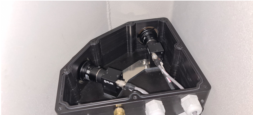
Figure 7.2: The camera housing which each camera pair is mounted in
