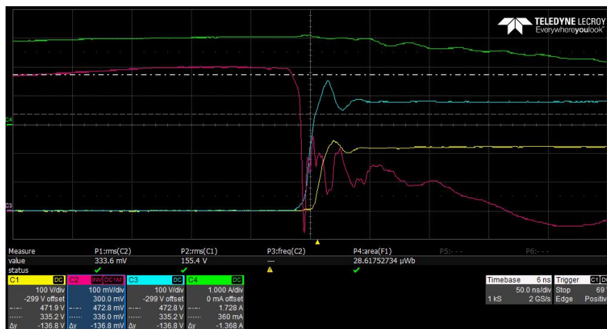
Figure 5.60: Improved voltage distribution as additional snubbers are added.
