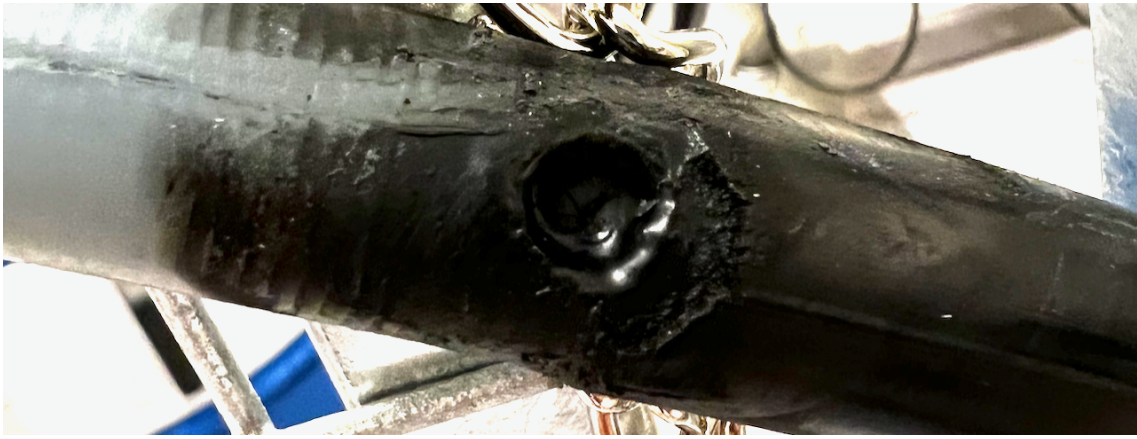
Figure 18: Picture of a breakdown in the termination
