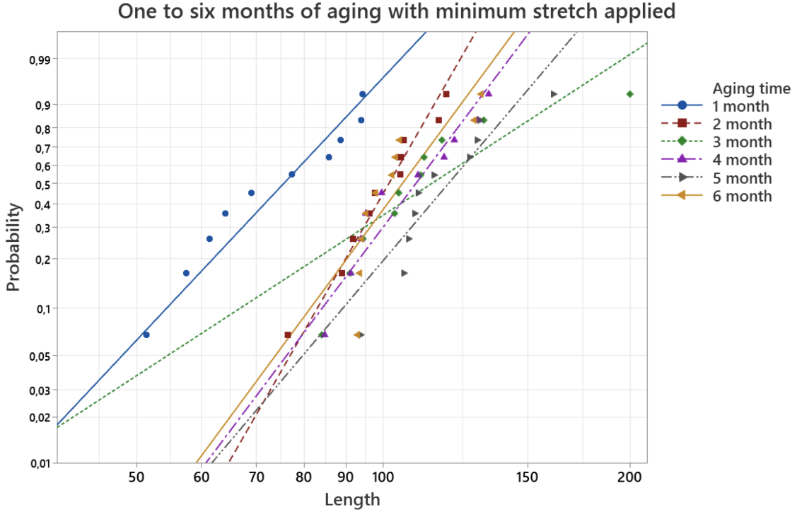
Figure 41: one - six months of aging with minimum stretch presented in Weibull probability plot
