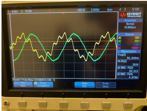
Figure 30: Without coil connected, the green signal is voltage and the yellow signal is current
