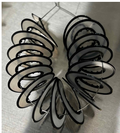
Figure 36: Picture of helically cut insulation.
