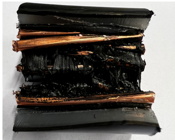
Figure 54: Picture of one of the test-objects cut open to confirm that there are strand-fill between gaps of the conductor strands
