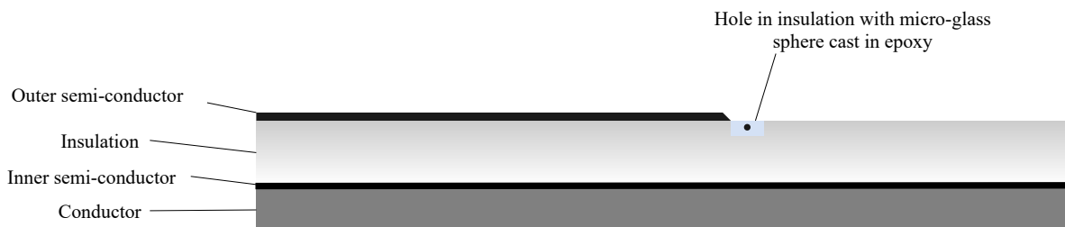
Figure 3.26: Principle of defect implementation of a micro-glass sphere in the cable insulation sealed by silicon or epoxy.
