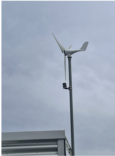
Figure 4.6: Location of the wind measuring unit, placed on the pole of the wind turbine.
