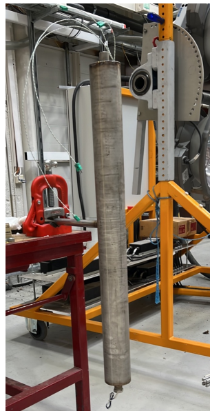
Figure 4.52: The test rig without insulation, mounted on a table using a clamp.
