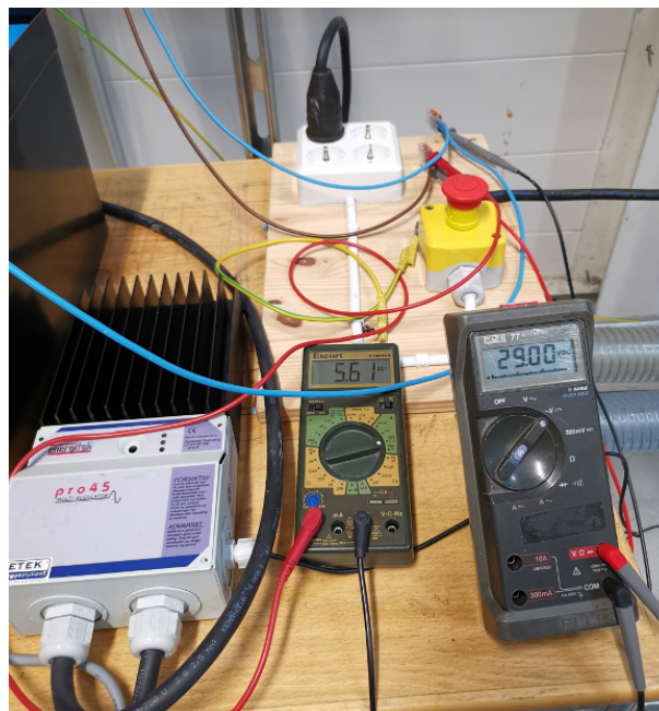
Figure 4.4: Multimeters connected to the solar array, voltage is measured to the right and current to the left.
