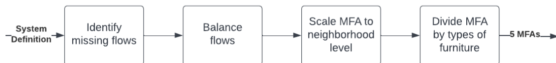
Figure 4 Steps taken to create the MFAs for 5 categories of furniture in the neighborhood
