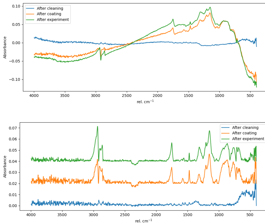
Figure 4.2: FTIR spectrum for steel sample coated with ODTMS After cleaning, after coating, and after the experiment. Raw spectra (top) and baseline corrected (bottom).
