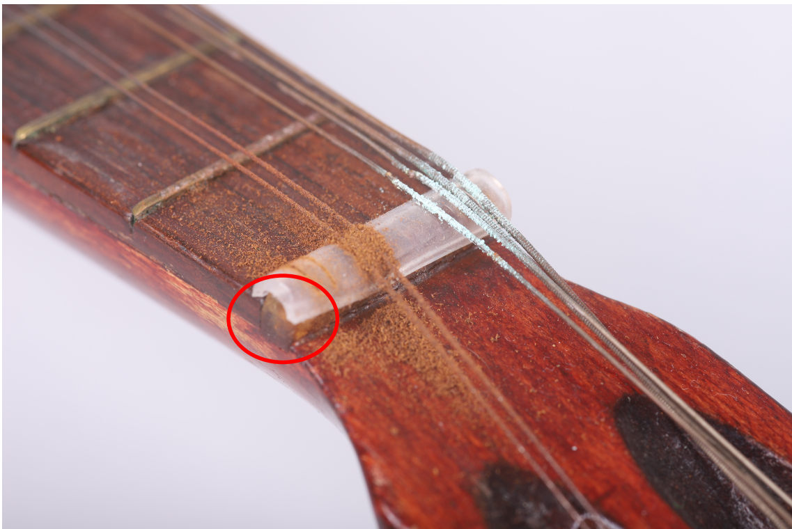
Figure 1.4: Image of the mandolin-banjo instrument with increased magnification in which the corrosion occurring at the instrument nut is indicated by the red circle. Ringve /Rockheim music museum.
