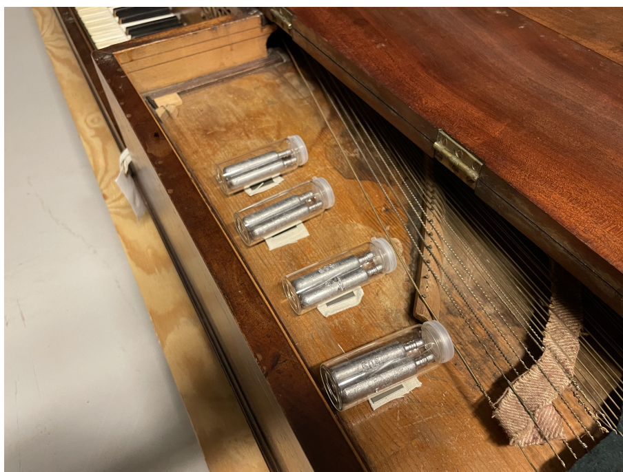
Figure 3.3: Steel and fabric weighted down by lead weights inside square piano in the storage facility of the museum. The samples were each prepared with different coatings: ODTMS, ODP, SA and a final uncoated sample.
