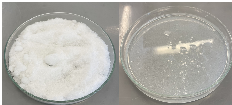
Figure 3.5: A saturated salt solution comprising of calcium nitrate tetrahydrate ( \text{Ca}(\text{NO}_3)_2 \cdot 4\text{H}_2\text{O} ) and water was prepared to enable control of humidity inside the desiccator. The image on the left shows the petri dish prior to the addition of water, and on the right the obtained saturated salt solution is shown.
