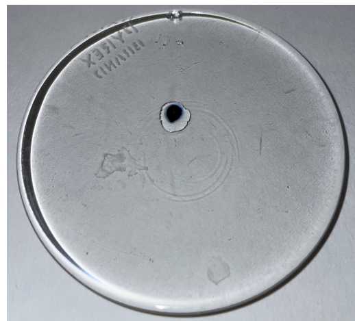
Figure 4.19: Diphenylamine spot test of sample material taken from the cellulose nitrate scratchplate showing a dark blue color.
