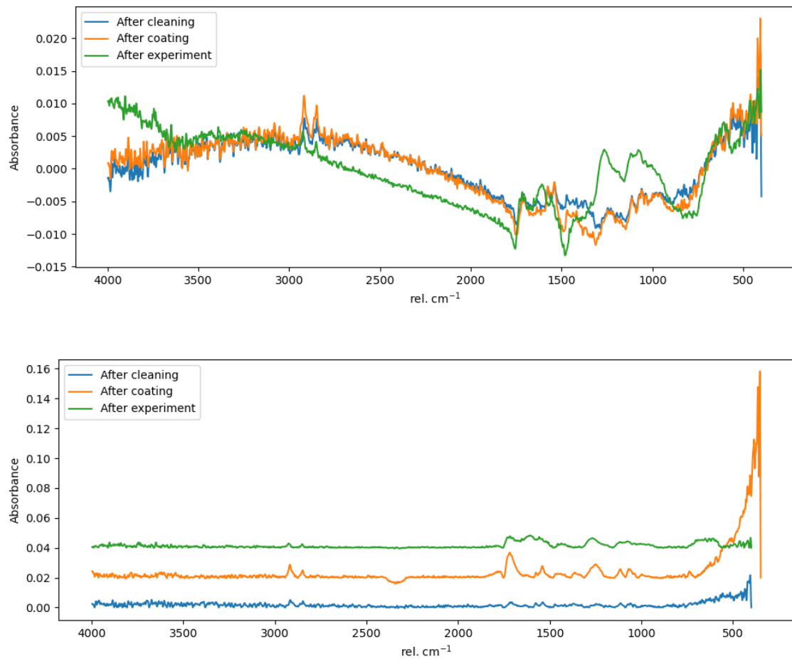
Figure 4.3: FTIR spectrum for steel sample coated with SA After cleaning, after coating, and after the experiment. Raw spectra (top) and baseline corrected (bottom).
