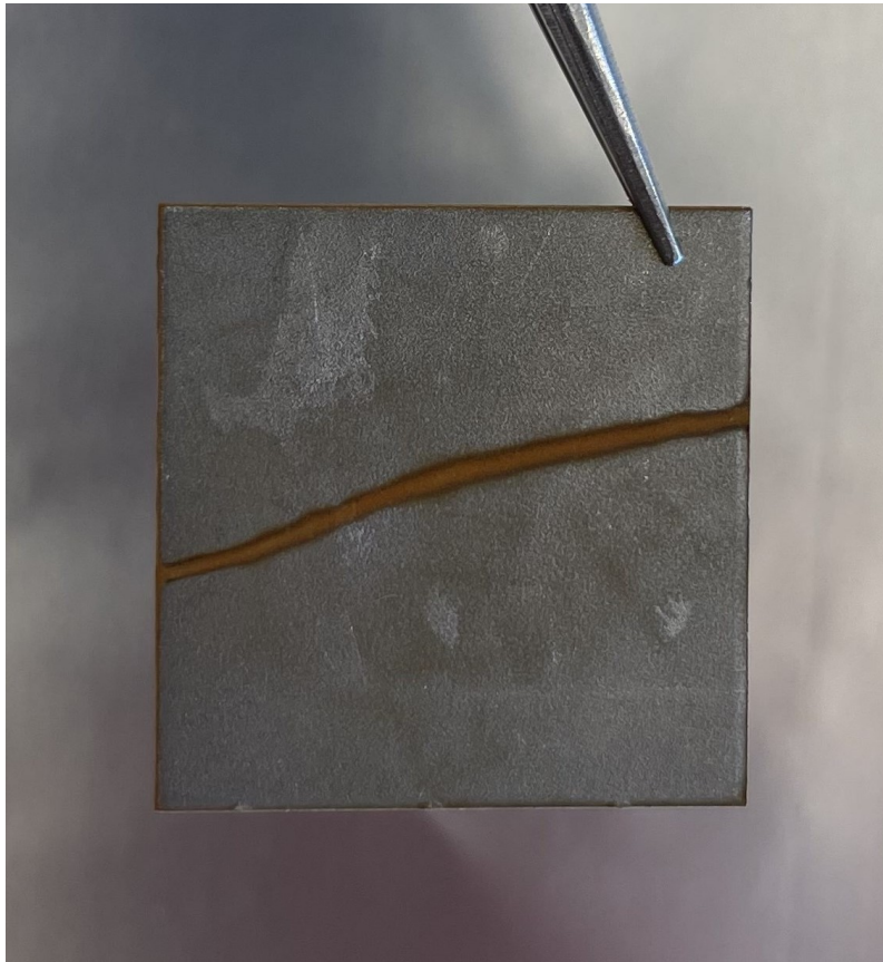
Figure 4.24: SA-tol Steel sample after two weeks of contact with cellulose nitrate scratchplate. A line of corrosion goes across the sample which coincided with a large crack in the cellulose nitrate plate.
