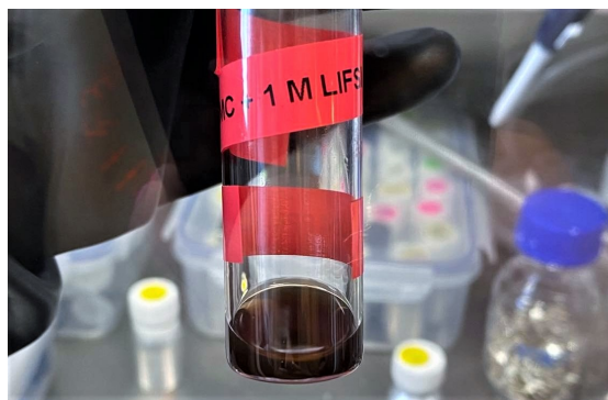
Figure 4.26: Picture taken of the FEC and water containing electrolyte
