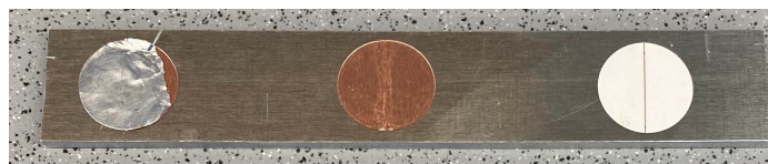
Figure 3.3: Method used to attach the Al samples onto the steel plate. Where the entire procedure of sticking the Cu tape to the plate, exposed Cu tape and the attached sample can be seen from right to left.
