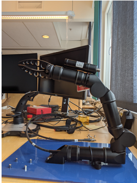
Figure 6.8: Reach Alpha 5 underwater manipulator.
