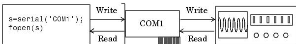
Figure 2.6: Illustration of serial port communication.
