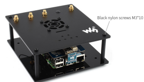
(g) Step 7: Assemble the top cover and fix with screws.
