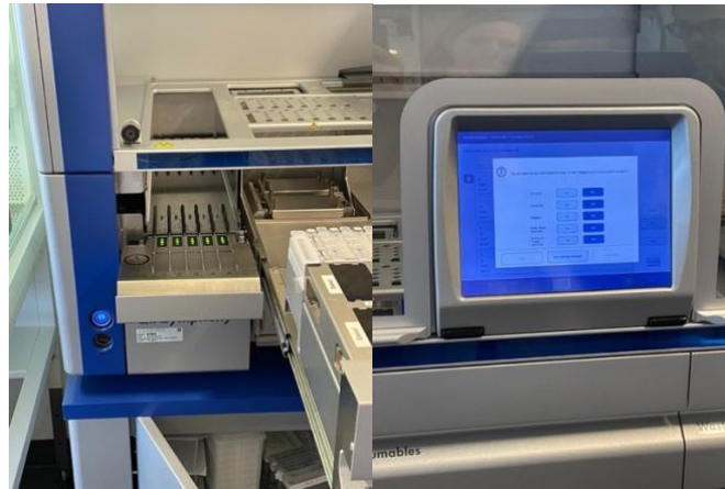
Figure 17: Placement of racks and touch screen
