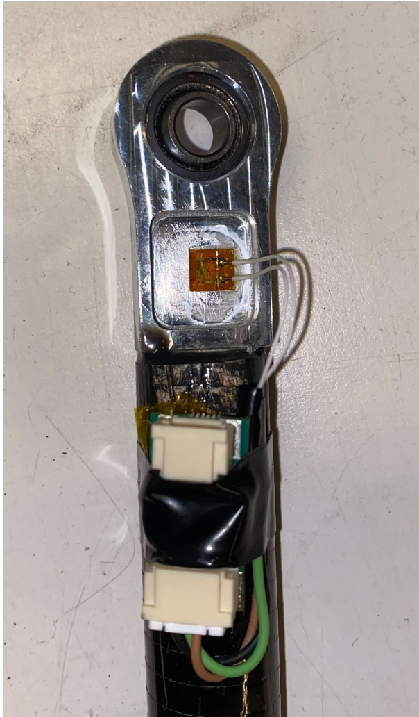
Figure 3.11: Strain gauge and amplifier mounted on the A-arm.
