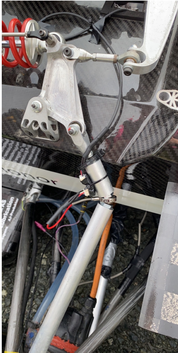
Figure 3.7: Buckled front right push rod on the 2019 car, Nova.
