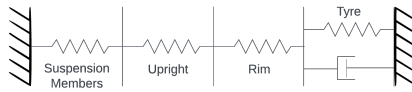
Figure 2.2: Simplified compliance model with the monocoque on the left end and the ground on the right end.
