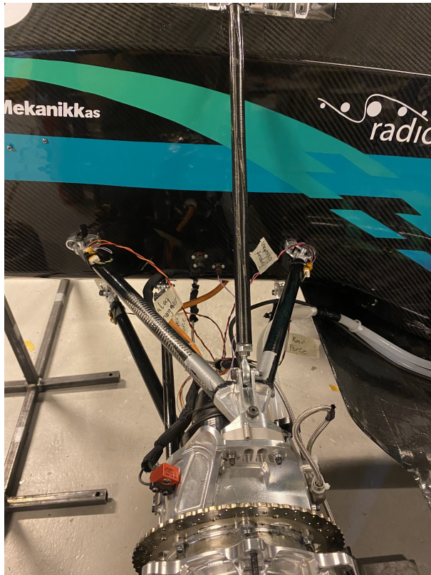
Figure 3.12: New A-arms mounted on Aurora.
