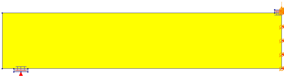
Figure 7.4: Model of three-point bending test
