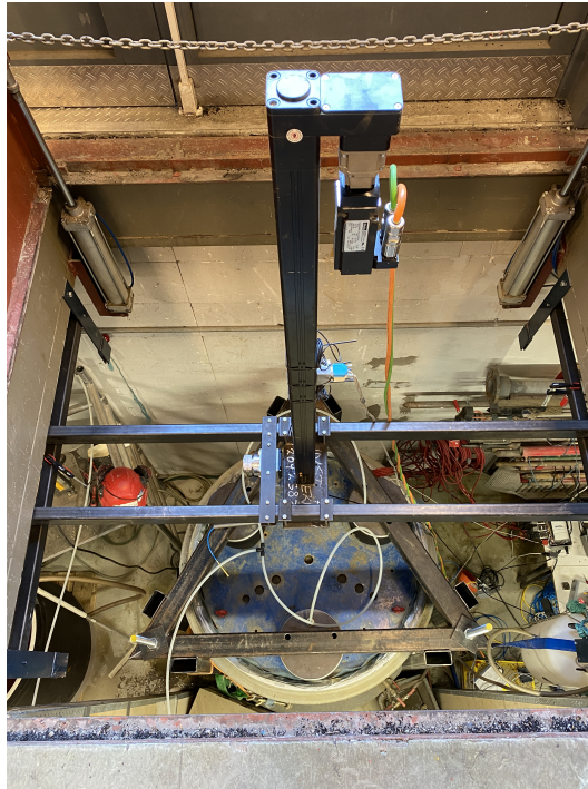
Figure 3.10: The actuator installed on metal frames to push the CPT through the sand sample at a constant rate of 15 mm/s.
