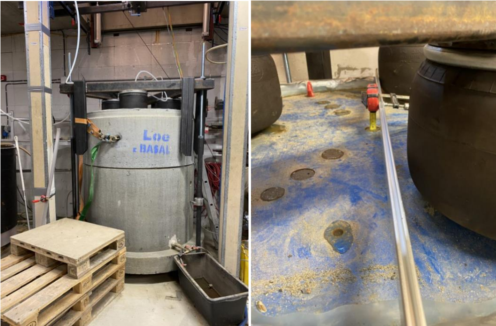
Figure 7: The loading frame is installed, and new measurements of the height are taken.
