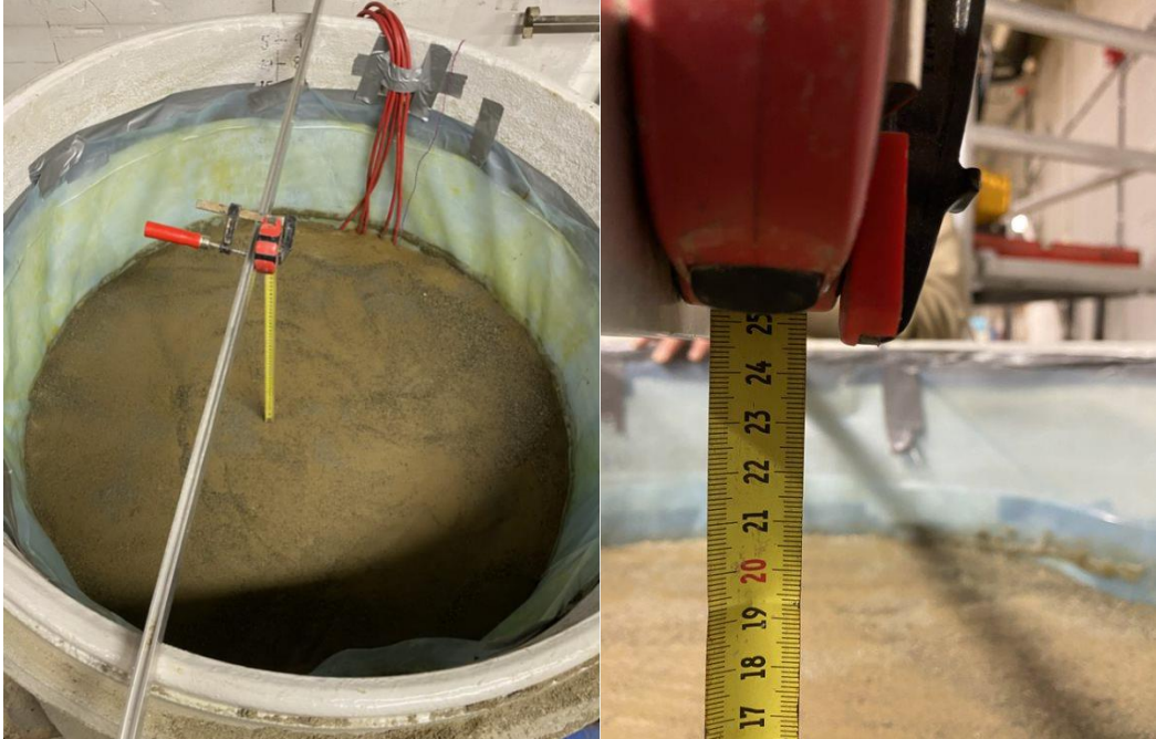
Figure 4: Water is emptied to achieve even compaction. The height is then measured.
