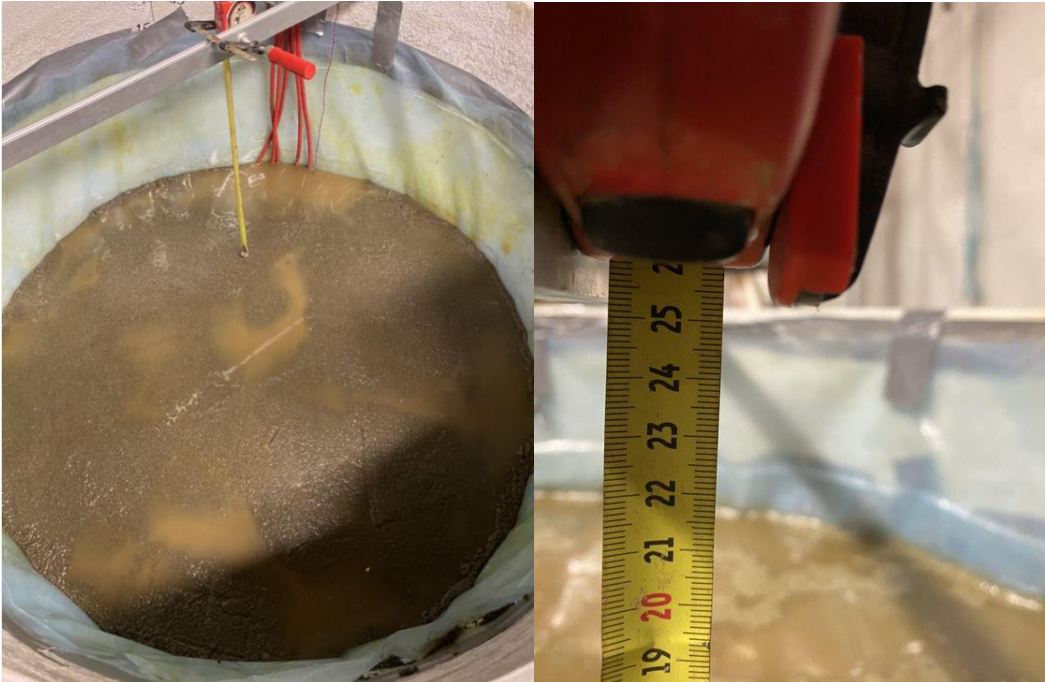
Figure 3: The sand sample is saturated with water and the sample height is measured with each step.
