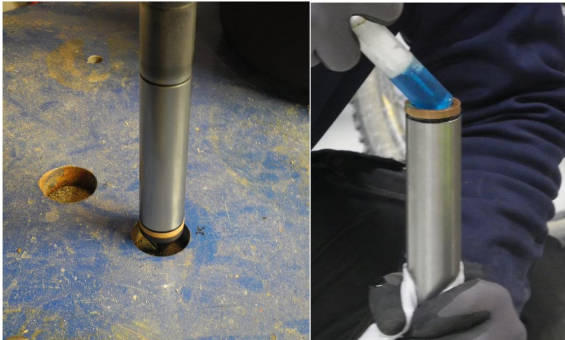
Figure 9: Cone penetration testing is performed for each section, 1, 3a, 3b, 3c, and the cone is saturated between each test.
