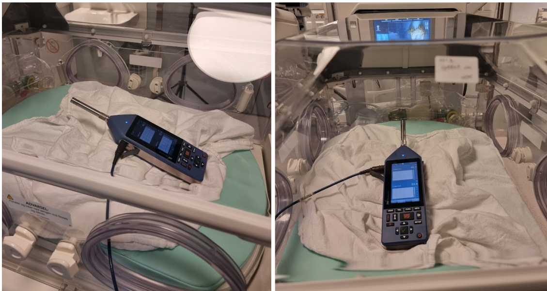
Figure 12: Microphone setup during measurements of sound pressure levels inside of an active incubator.
