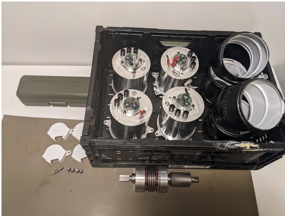
Figure 5.5: Four motors finished mounted and calibrated.
