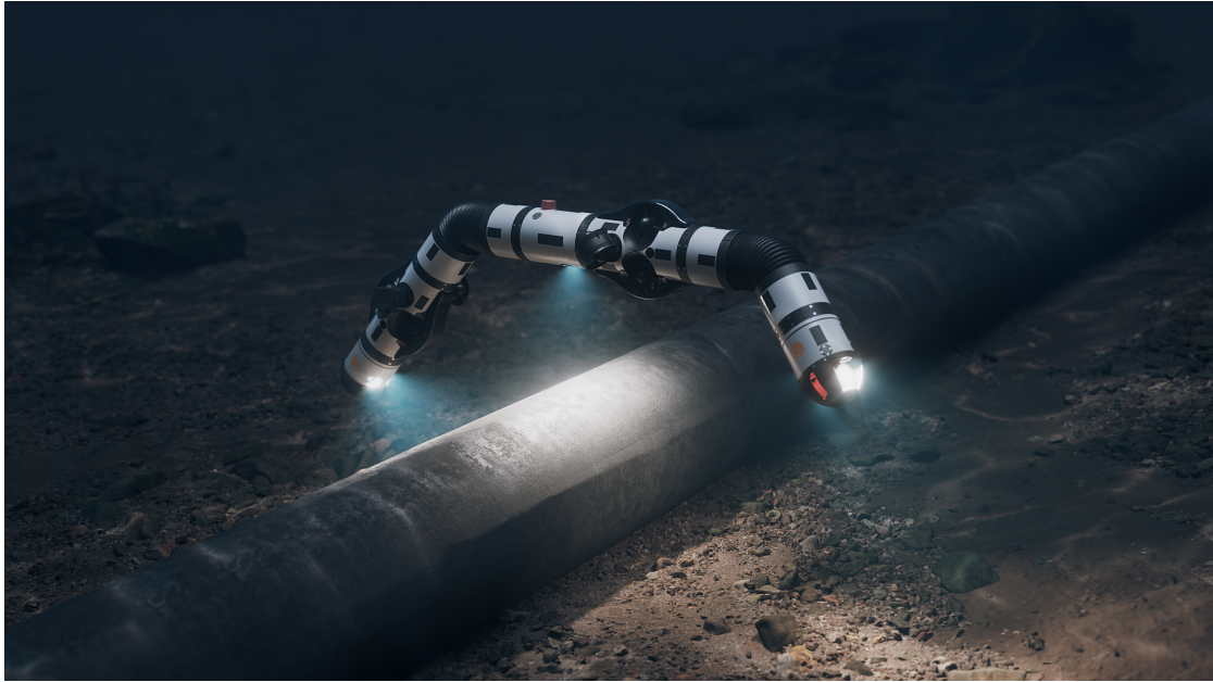
Figure 1.1: Inspection of underwater structures using the Eelume robot. Image courtesy: eelume.com.
