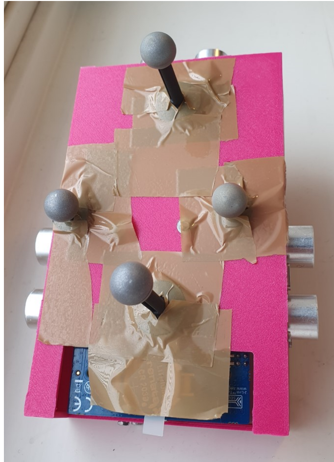
Figure 13: Placement of spheres for the three dimensional test
