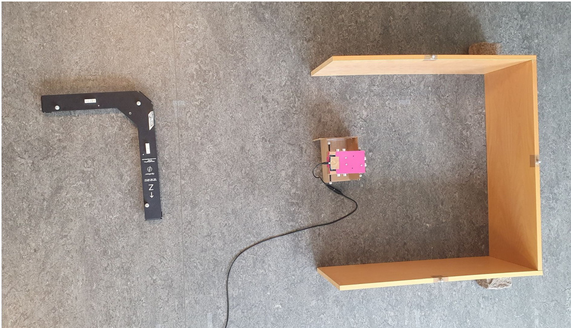
Figure 12: Calibration square to the left, walls and casing with sensors to the right
