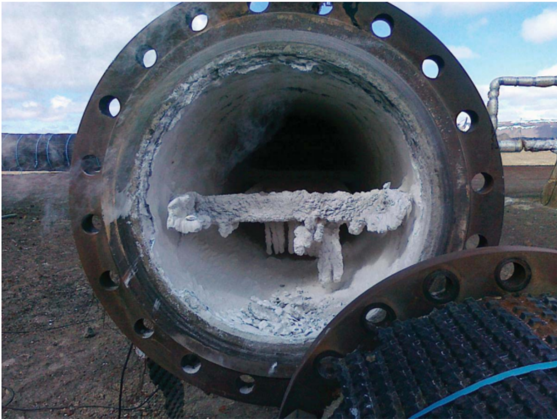
Figure 1.1: Illustration of the deposition of silica dust in a silencer line from the IDDP [8]
