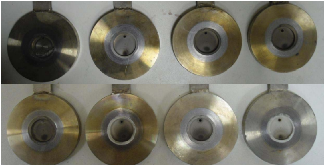
Figure 6.3: The scaling of silica on the different orifices in the experiment 1 of the IDDP cascade test
