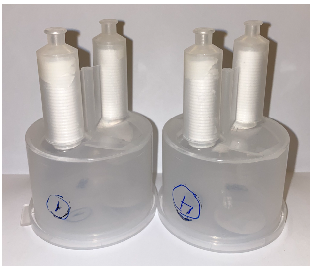
Figure C.3: Photo of the centrifugal Centricon filters with accumulated SBG oligomers
