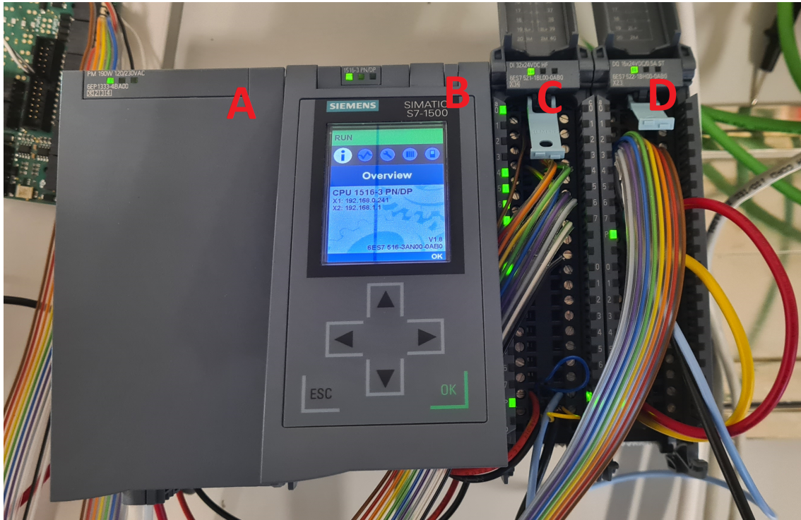
Figure 2: Siemens S7-1500. A) Power supply unit, B) CPU (1516-3 PN/DP), C) Digital Input module (DI 32x24V DC), D) Digital Output module (DQ 16x24VDC/0.5A ST)
