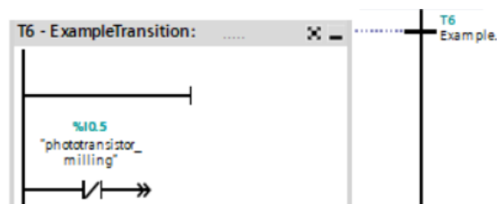
Figure 9: Unclosed branch in transition leading to error.
