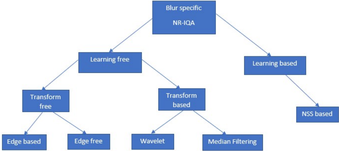
Figure 3.7: A comprehensive categorization of blur-specific, no-reference image quality evaluation techniques, including learning-free and learning-based techniques.
