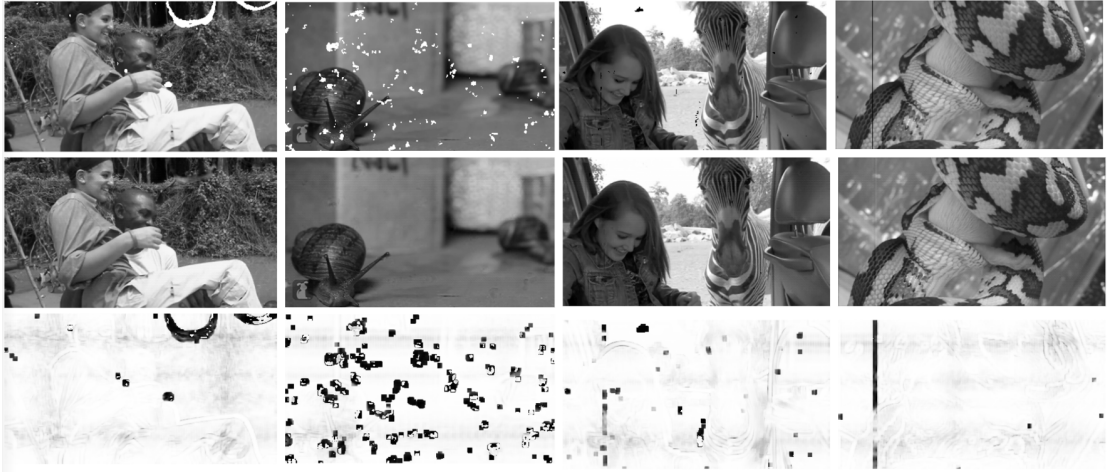
Figure 5.7: The first row represents the masked frames that are artificially generated and the second row refers to the corresponding restored frames by the proposed model trained using the video inpainting approach. The last row depicts the SSIM difference map among the masked and restored frames
